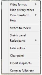
**Video format:** Allows the user to select which of the cameras video streams (which format/resolution) they wish to view.
