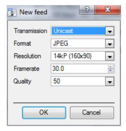
**Transmission** will show the transmission type **Format** is the compression format used by this stream. Click the drop-down menu to choose the one you desire. **Resolution** is the amount of pixels in the image. **Framerate** is the amount of frames recorded per second **Quality** defines how lossy the compression of the image is.
