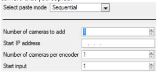
**Start IP Address** will determine the IP address of the first new camera that you are adding. The IP addresses will be incremented from here. (So make sure you have no used IP addresses in this range.)
