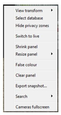
**View transform:** Allows you to transform images for cameras with special lenses. (E.g. 360 degree cameras.)
